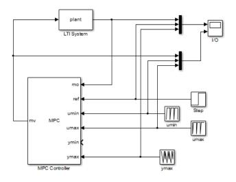
If any of these inports are unconnected, they are treated as unbounded signals. The corresponding variable in the mpc object must also be unbounded.
