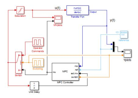
If the external MV option is inactive or the ext.mv inport in unconnected, the controller assumes that its MV output is used in the plant without modification.
